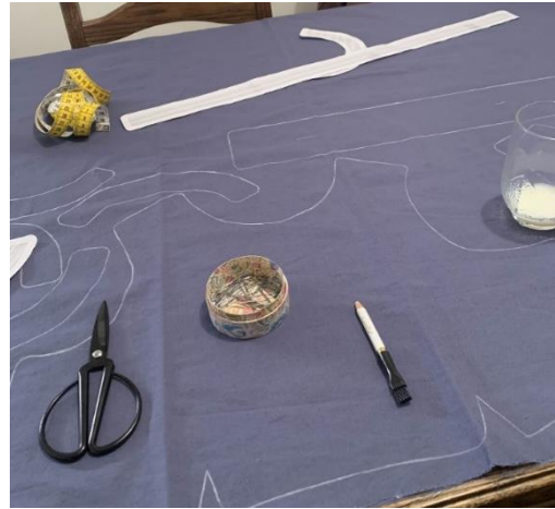
Figure 27. Marking on the fabric where to cut.
