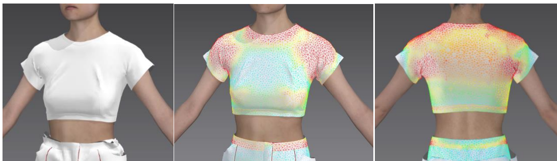
Figure 23. The top (left) and the top with a strain-map showing the fit (middle, right)(red = stretched fabric, blue = relaxed fabric).
