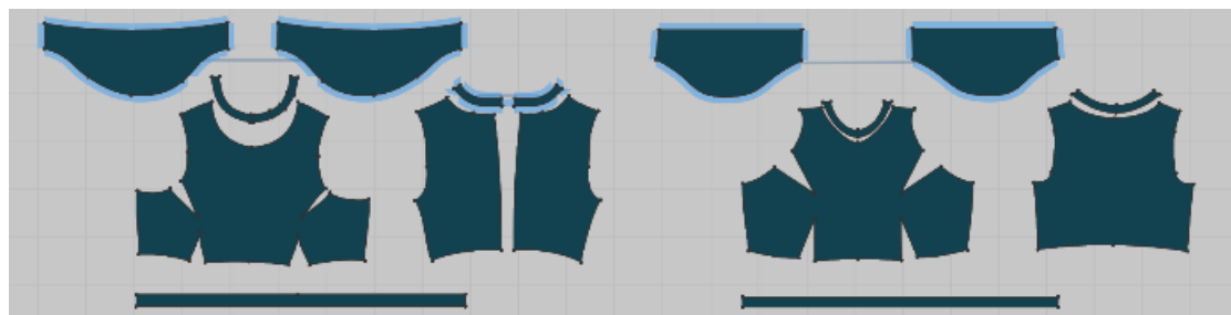
Figure 9. The adjusted sewing pattern (left) and the original sewing pattern (right).
