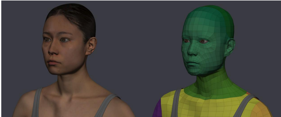
Figure 21. Highpoly mesh (left) and lowpoly mesh (right).
