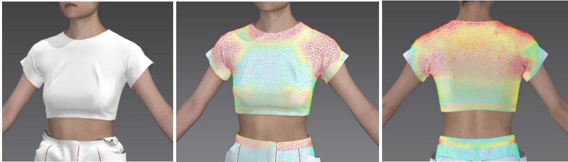
Figure 8. The top (left) and the top with a strain-map showing the fit (middle, right)(red = stretched fabric, blue = relaxed fabric).
