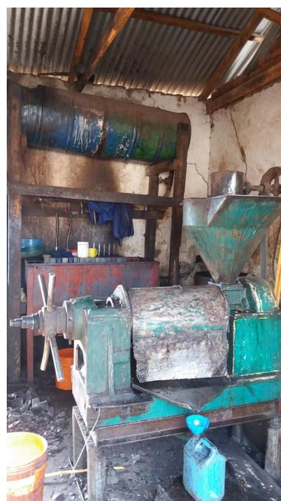
*Illustration 3: Sunflower oil expeller (front) and filtering equipment (back) at a processing plant in Gallapo, 2016-02-25.*
