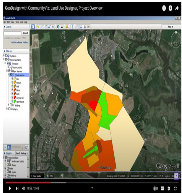
Image: View of the Communityviz software that allows the user to visualise maps together with other relevant variables such as land use, population density, infrastructure, and environmental data.
